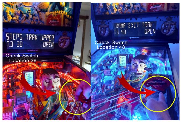
The three switches should match the examples above in the display. If they do not wires will need to be removed and routed to the correct switch as shown in the above Pictures. Switch 38 is the upper switch in the wire ramp and switch 48 is the lower Switch in the wire ramp. This would also be a good time to verify other switches on the game and verify that all switches read properly on the display.
